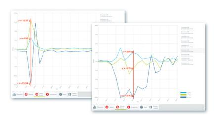
The course of a shock can be traced in milliseconds and per axis. As shown here in detail, the amount of acceleration per axis is not the only relevant factor, but also the duration of the shock. This allows serious damage to be detected.
